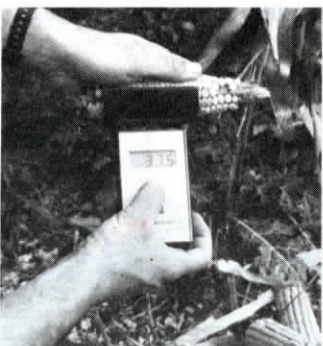
Tester checks moisture of corn on cob. Can even be used on corn still on the stalk with the husks on.
