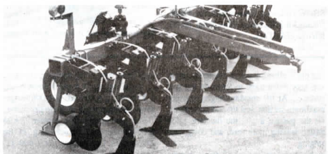
The 18-in. coulters are equipped with scrapers, cast hubs and dual re-lube bearings.
