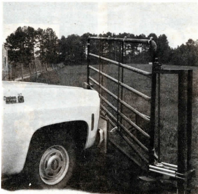
As you drive through, vehicle's bumper pushes against "bumper pad" attached to the gate. After 4 ft. of travel, the gate swings open automatically.
