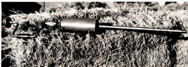
Threaded coring tube easily screws into tightly-packed bales.
