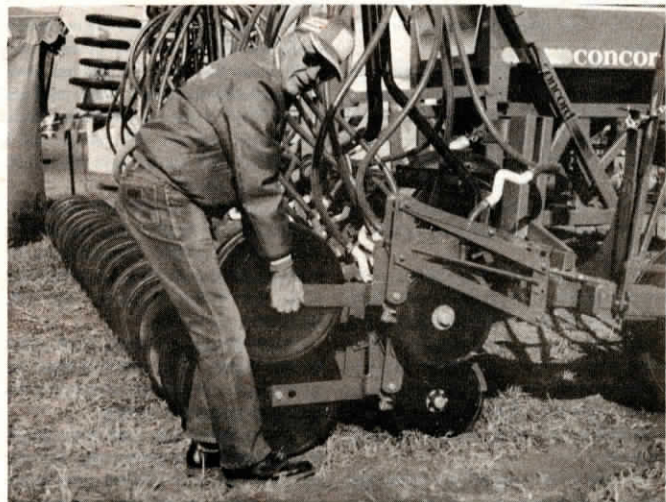
Each row unit has a full 22-in. range of independent up and down motion.
