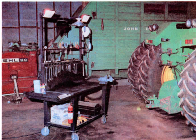
Wheeled workbench is equipped with pair of halogen lights and electrical outlets.
