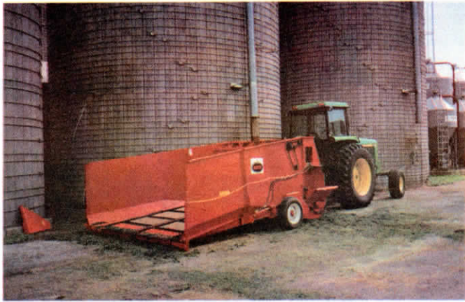
Conveyor is equipped with an up-front side opening, allowing two different silages to be blended and loaded into silo simultaneously.
