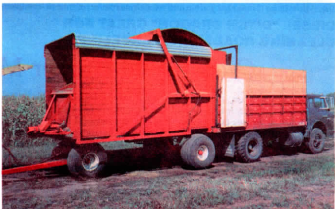
"Push off" box mounts on truck and is used with push-off chopper wagon.
