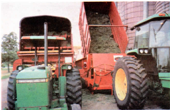
Loads of freshly-chopped silage are dumped onto 12-ft. long self-tending conveyor which feeds material into attached blower.
