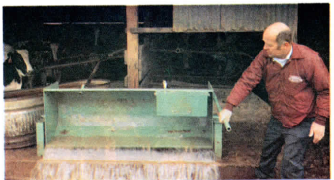
Hinged tank is equipped with a dump handle for fast, easy cleaning.
