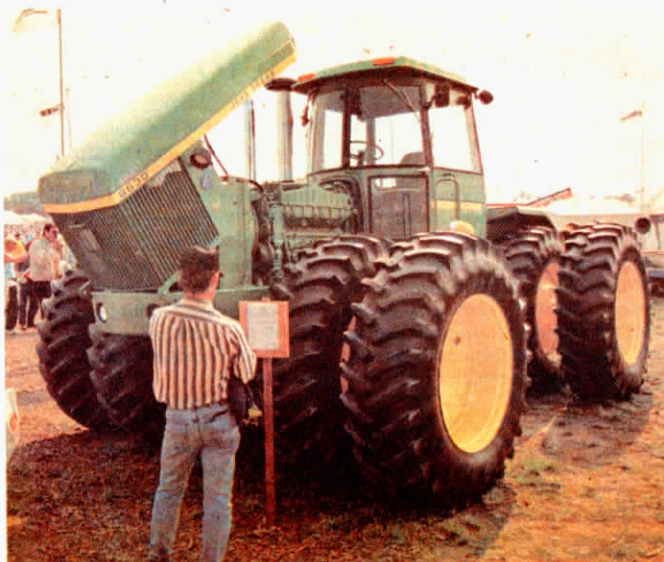
One modification Kinzenbaw makes when repowering Deere 4-WD's is to move the exhaust and air cleaner stacks off to the side so the hood can be made to hinge.
