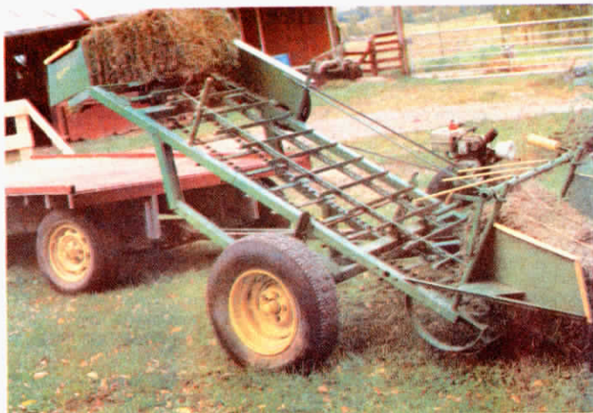
The lower front end "floats" along the ground on a curved skid plate and the entire unit pivots up and down on the axle.
