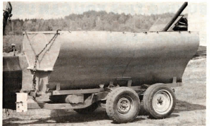
Davidson salvaged the front halves of two identical car frames and welded them together nose-to-nose.
