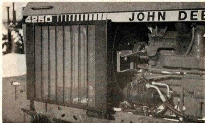
Scroll-like screen is continuously rolled back and forth onto rollers at either side of unit (hidden in photo by end guards).
