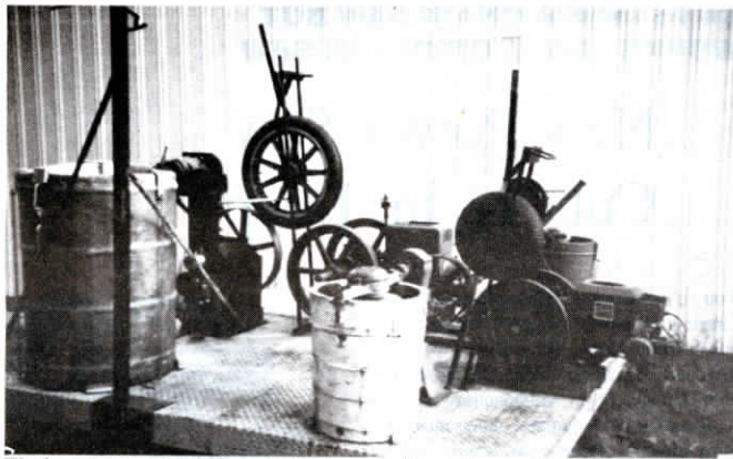
The ice cream maker is operated by two gasoline engines and consists of one 25-gal. and two 5-gal. units. Rubber tire "clutches" drive each unit.
