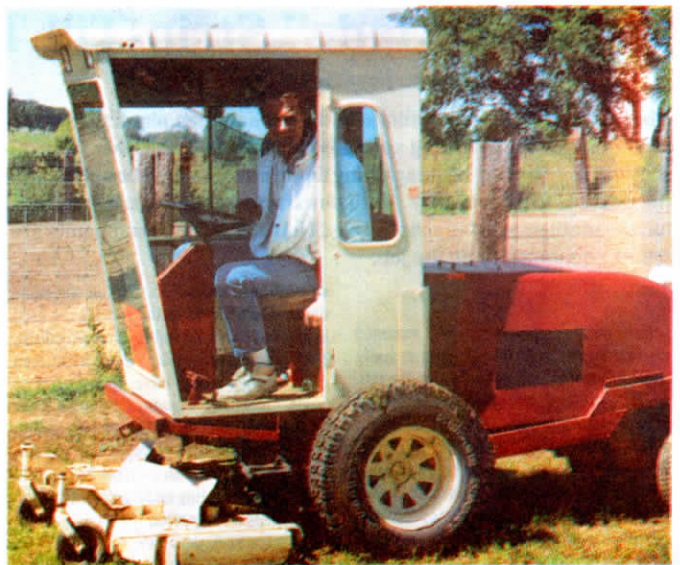
Tractor steers at rear like a combine and has front-mount deck.
