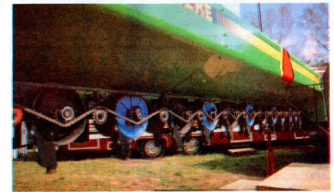
Kinze brush-type seed metering units bolt on in place of drill’s original metering units.
