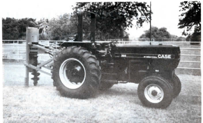
Digger is equipped with opposing cylinders, located above the gearbox, that use the weight of tractor to apply down pressure for high-speed drilling.
