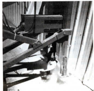
With special cutting tip, "down pressure digger" will dig through concrete.
