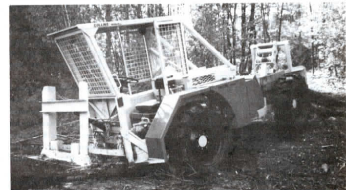
There's 17 in. of clearance for rocks and stumps, yet the center of gravity is low.
