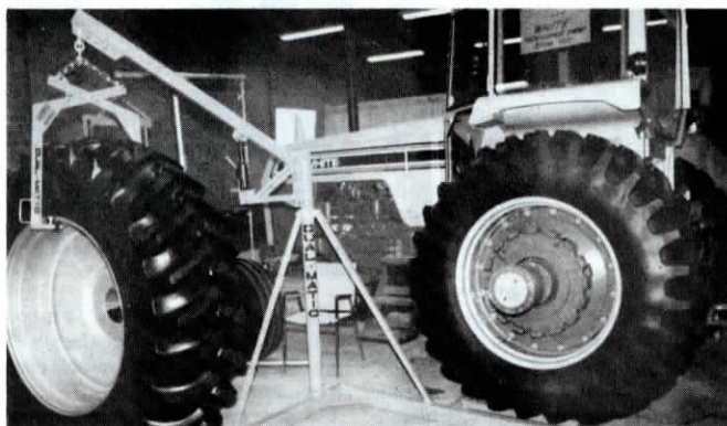
The swing-away lift arm is mounted on a pedestal that consists of two brace arms and a drive-on stand. Any 3-ton hydraulic jack can be inserted under the lift arm.
