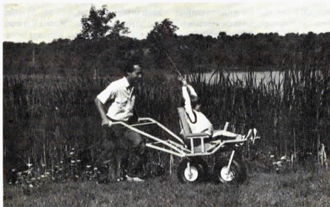
The 54-lb. wheelchair resembles a large wheelbarrow and rides on balloon tires.
