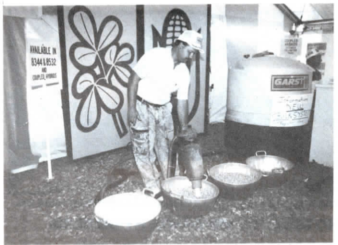
Seed is conveyed from 35-bu. polyethylene seed tank to discharge nozzle which is used to fill each planter hopper. Seed drops out of the nozzle by gravity.
