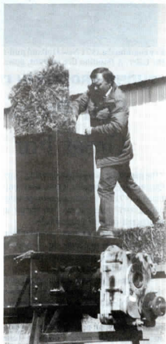
Anderson hand-feeds bales into the grinder's 20-in. sq. hopper. Fifty offset knives, powered by a tractor pto, grind the hay at 20 rpm's into 3 to 5-in. long wafers that drop out bottom of grinder.
