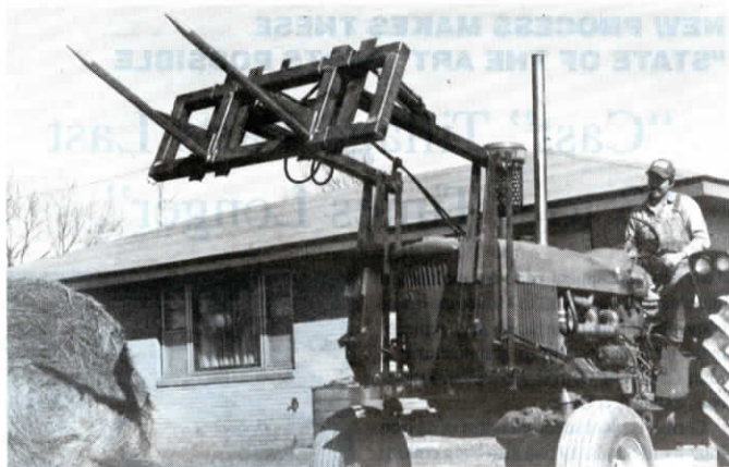
Front end bale-loading spear features two independent bolt-on scissers that raise and lower a twin-pronged spear for loading and unloading big bales onto flatbeds.
