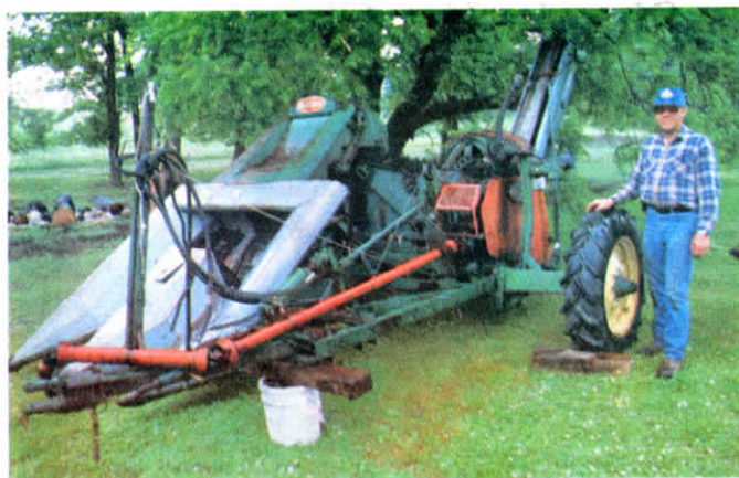
Peterson hinged tongue on picker, installing a hydraulic cylinder (at center in photo) which reacts to "row finders" on snout. He also extended outside wheel on picker by 2 ft. to run between ridges.
