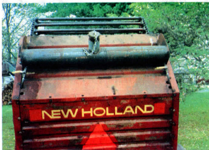
Kirby attached steel pipe reservoir to baler endgate with hoses at either end to apply constant flow of oil to chains.
