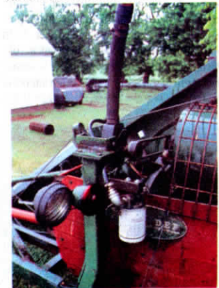
Power steering pump provides power to hydraulic cylinder on tongue. It's driven off pulley on picker fan.
