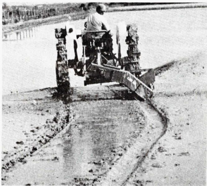
Above photo shows ditcher making 6 by 12 in. ditch in field for pothole drainage. Cutter head on D60 is offset 32 in. from drive shaft. Another model (D80) with 40 in. offset is also available.
