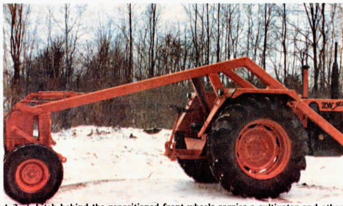
A 3-pt. hitch behind the repositioned front wheels carries a cultivator and other implements.
