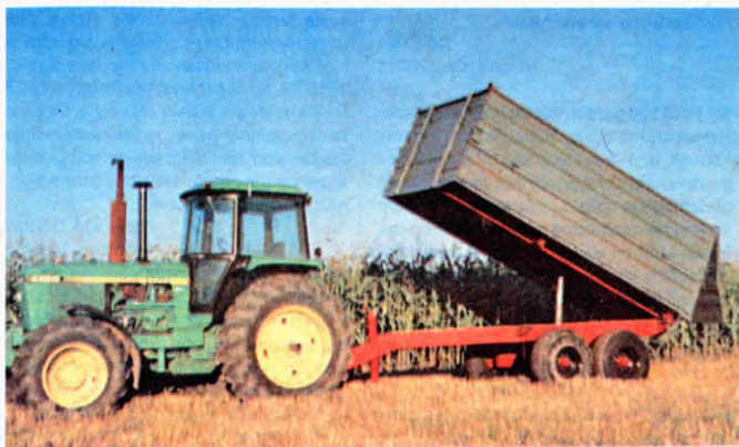
The new 12-ton capacity wagon box can be truck or trailer-mounted.
