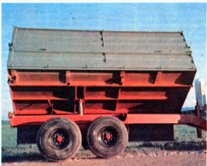
To switch from rear to side dumping, or vice versa, you simply switch two pins.
