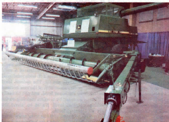
New kit extends hitch and driveshaft to make room for direct-cut heads on pull-type machines.
