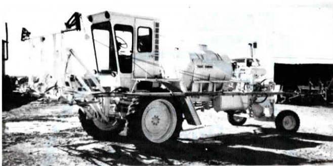
Corder mounted the primary components of an IH 715 combine on a truck frame.
