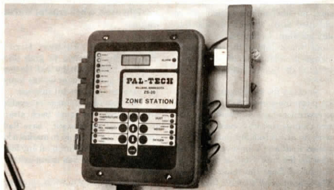
Control panel lets you program desired levels for temperature, humidity, ammonia and dust.
