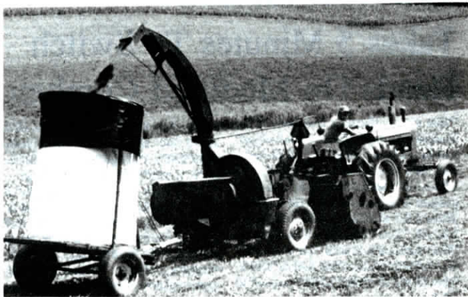
Full bags are tied, then dumped onto the ground by pulling a pin on the hinged cage.
