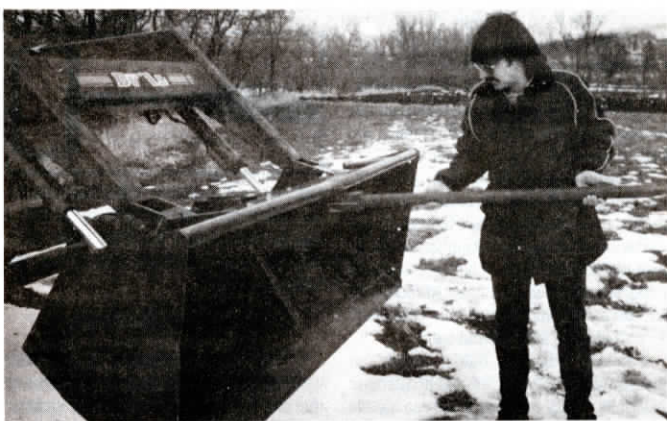
Steel bracket bolts under top plate of bucket, close to front edge. Spear is secured inside bracket by 3/4-in. dia. steel pin.
