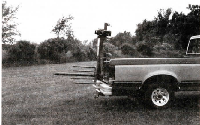
Bale unroller bolts to steel frame that mounts at back of pickup box. Bale spear mounts on plate that's rotated by 2 1/2 hp electric motor wired to pickup battery.
